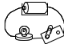
A switch can be used to create a break in a circuit.
